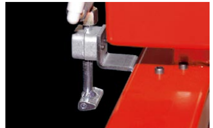
Air jet for separating the sheets
